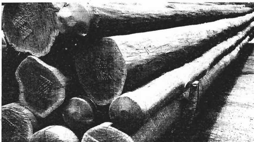
Hardwood poles freshly removed from the treatment cylinder following vacuum pressure impregnation with PEC, our new, cleaner cresate-based preservative.
