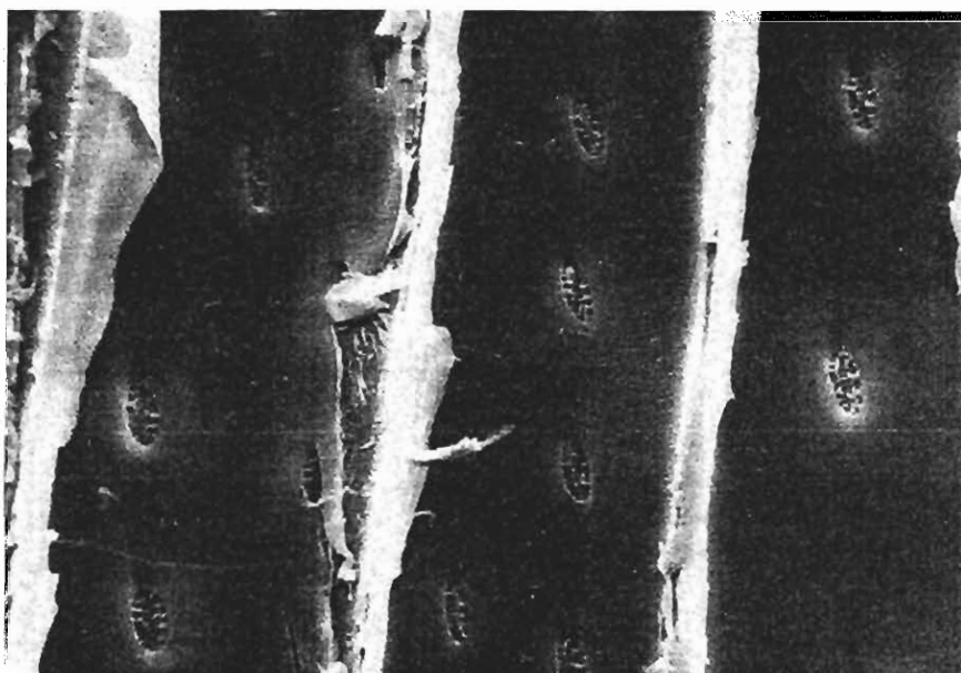
Investigating the structure of fibre pits will provide a better understanding of wood permeability (E. regnans fibres \times c. 1000 ).
