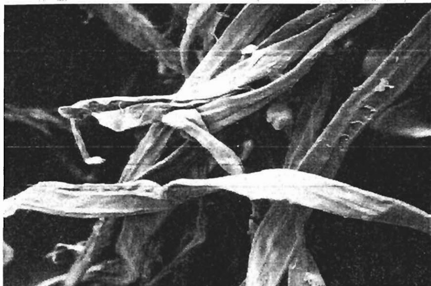
Fig. 2. A scanning electron micrograph of kraft wood pulp fibres
