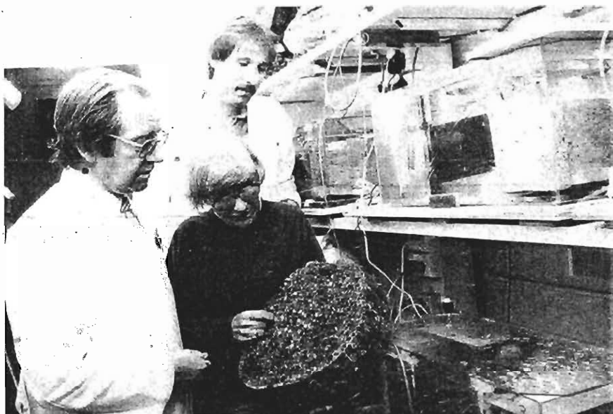
Professor Turner (centre) is discussing shipworm damage in a eucalypt pile with John Barnacle (left) and Laurie Cookson (right).
